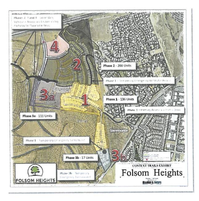
Below is the TM grading plan that shows the general location of proposed temporary EVA. By way of further detail the Winterfield cul-de-sac is roughly at elevation 600 and the other end of the EVA at the Phase 1 boundary is approximately elevation 700 proposed grade and approximately 720 existing ground. The EVA will connect at Winterfield and then will generally follow the existing ground and then transition to connect to Phase 2. The slope of the EVA will be between 10 and 12%.
