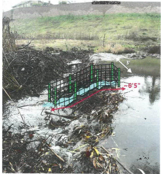
Figure 1. An example design of a notch exclusion fence placed in the Stonebriar Dam. The channels on either side of the lodge represent the main channel and should be targeted.
